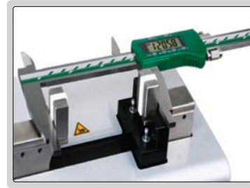
caliper zero setting and calibration
