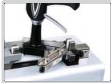
three-point internal micrometer zero setting and calibration
