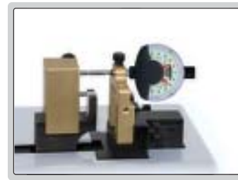
dial comparator zero setting and calibration
