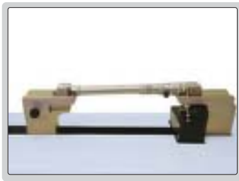
tubular inside micrometer zero setting and calibration
