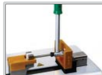
bore gauge zero setting and calibration
